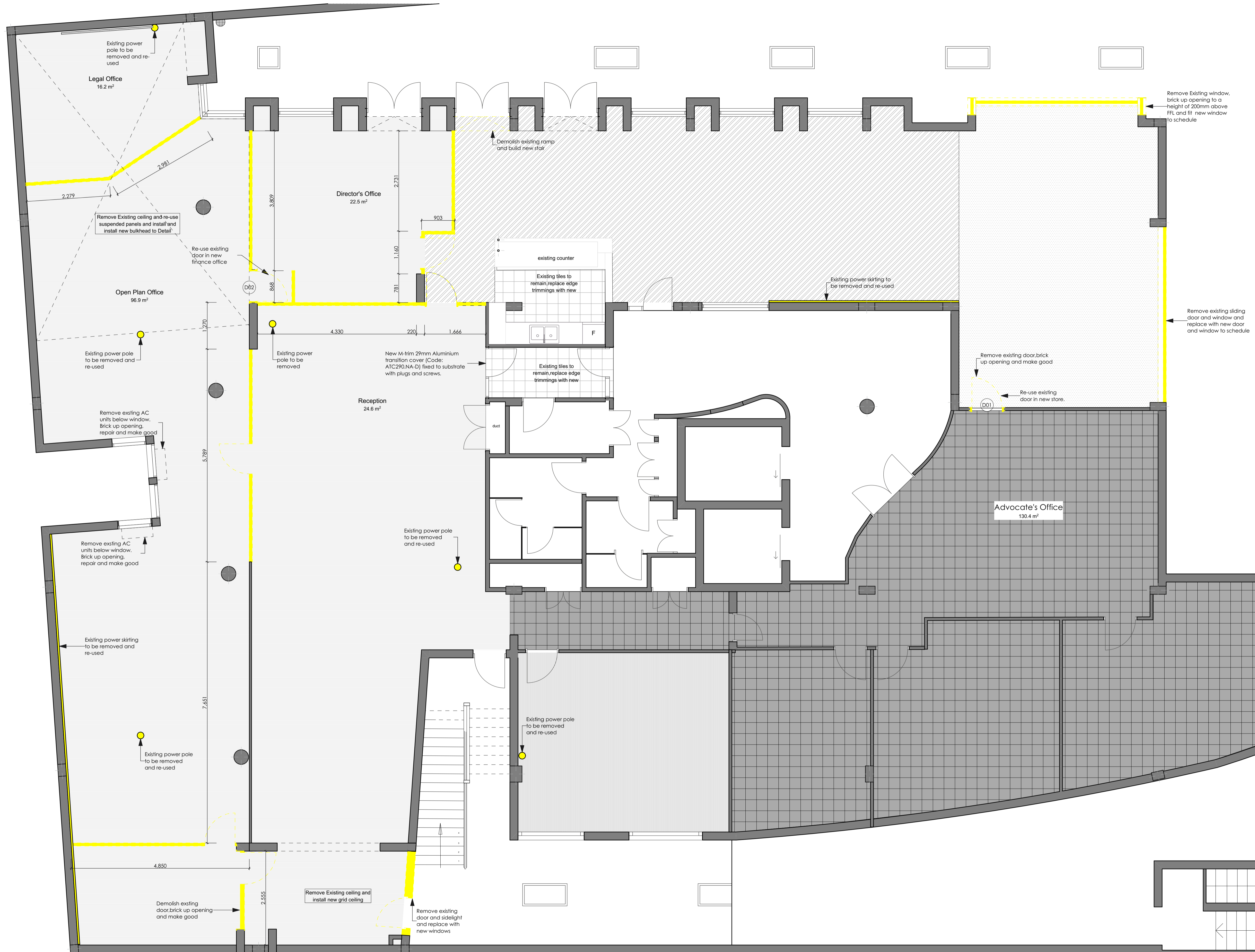
Demolition Plan Scale 1:50
