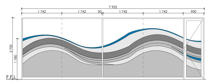
DOOR 7932 x 2700mm High Purpose made natural anodised aluminium door with sidelight as indicated.
